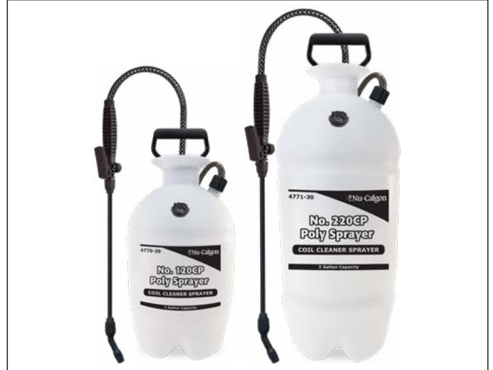
5. Pump plunger to compress air and create pressure in tank. Twenty strokes of plunger provides a good working pressure. As pressure drops during use, recharge with 20 or more pump strokes. More strokes will be needed if the tank is not full, or as the sprayer is used and the pressure drops.
